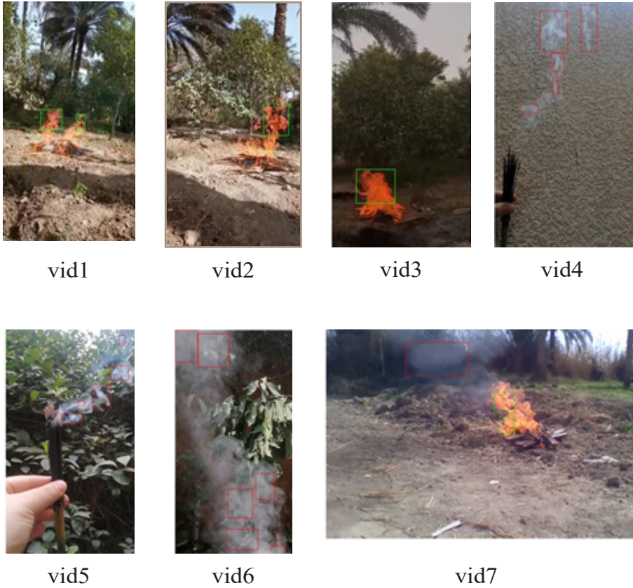
Figure:5, Test results of the real-time flame and smoke detection
